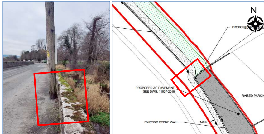
Figure 2-3 Drawing 11007-2014-D01 extract showing interface between road and proposed footway
