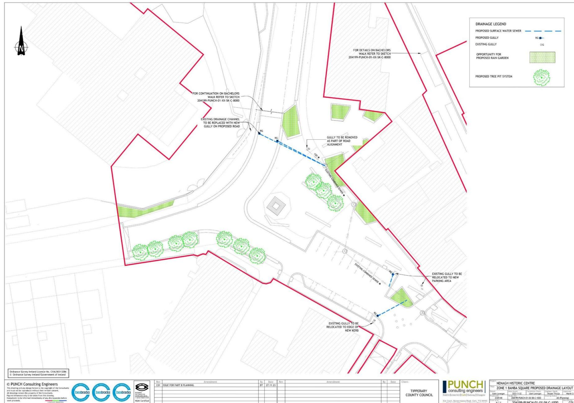
Figure 3-5: Proposed Stormwater Drainage Banba Square (NHCQ Zone 1)
