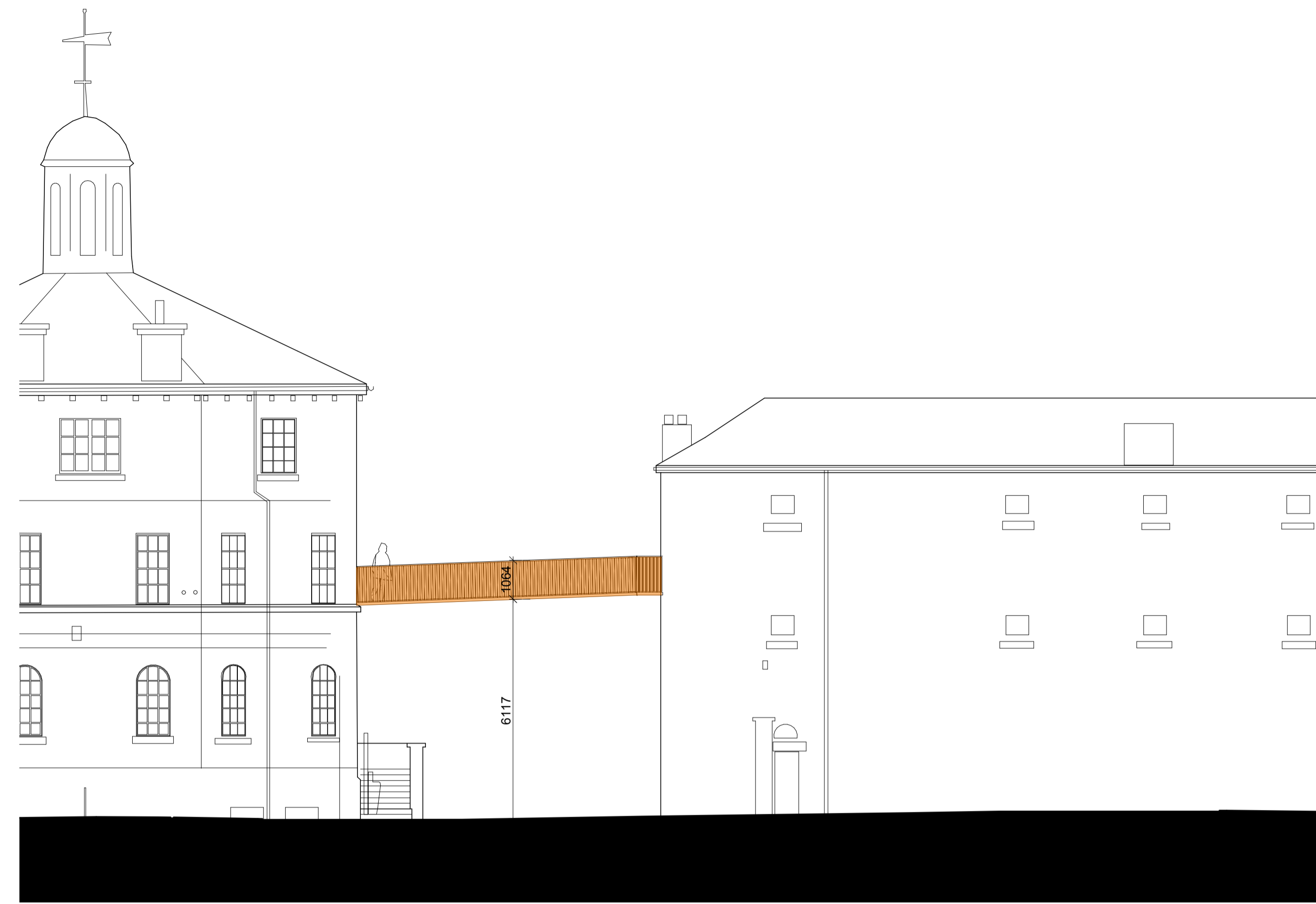
2 PROPOSED BRIDGE - WEST ELEVATION SCALE: 1:100
